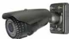
> **VD6860 Infrared video camera with Day&Night varifocal lens high resolution with mechanical IR filter**
